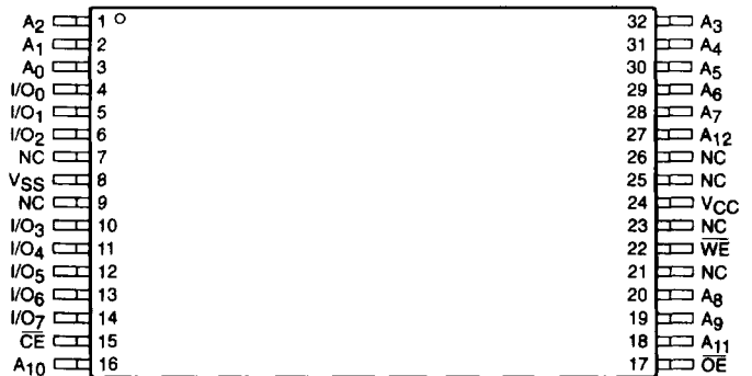
TSOP Top View (8mm x 14mm) (T14) TSOP Top View (8mm x 20mm) (T)
